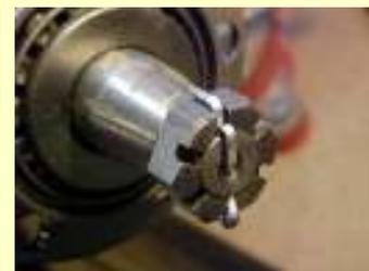
over the nut face and the other is over the shaft. This is what a properly installed Cotter Pin should look like. Finding castle nuts is not difficult, many hardware stores will have a good selection. Finding an appropriate bolt with a hole in it is another matter. Here is a little jig that I made for 3/8 inch bolts, to add a Cotter Pin hole. It is drilled and tapped to hold the bolt. There is a small hole
