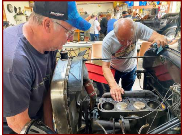
DeWayne prepped both sides of a new copper head gasket with copper gasket sealer.
