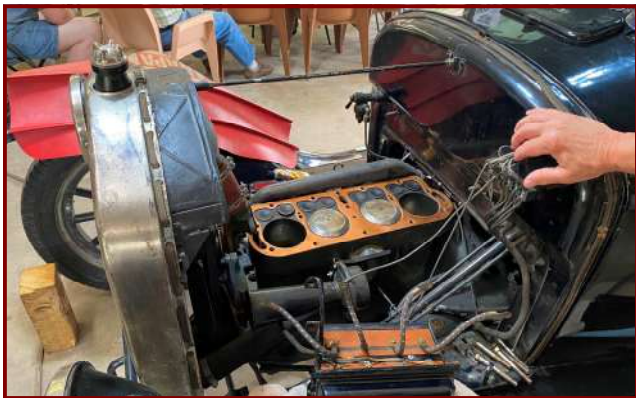
DeWayne prepped both sides of a new copper head gasket with copper gasket sealer.
