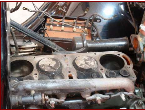
DeWayne prepped both sides of a new copper head gasket with copper gasket sealer.
